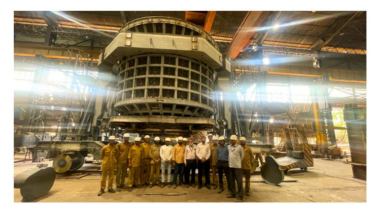
Mukand Limited, a Bajaj Group company and a leading manufacturer of Stainless Steel has been at the forefront of heavy machinery design & manufacturing for over six decades now.The company proudly announced the successful manufacturing of its first-ever Coke Bucket and Carriage, a critical component in the Coke Dry Quenching (CDQ) system.
