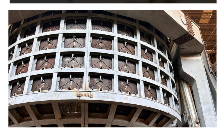
The Coke Dry Quenching (CDQ) process is an advanced and environmentally friendly alternative to traditional wet quenching. By through nitrogen circulation, dry cooling CDQ utilizing gas CO<sub>2</sub> emissions, conserves significantly reduces water. and enhances coke quality. This technology plays a pivotal role in mitigating environmental impact while ensuring greater energy efficiency in steel manufacturing.
