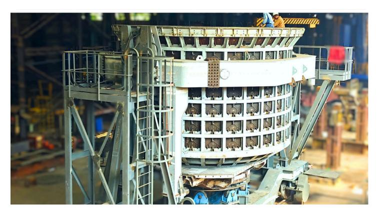
The Coke Bucket and Carriage system is a key element in the CDQ process, ensuring the safe and efficient transfer of hot coke (maintained at  $1050 \pm 50$  °C) from the coke oven to the CDQ chamber. The system consists of a rotary coke bucket that is transported via a coke bucket car, powered by an electric locomotive, and lifted to the top of the CDQ chamber using an elevator system.
