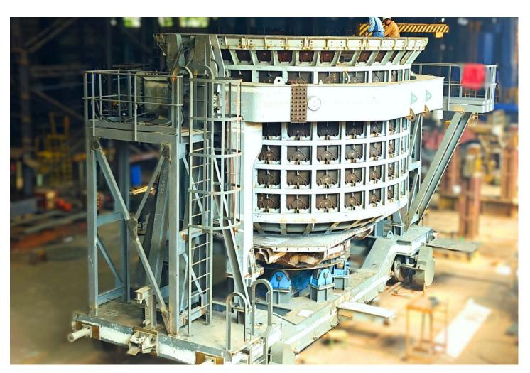
Bajaj Group company Limited, a Mukand and leading a manufacturer of Stainless Steel has been at the forefront of heavy machinery design & manufacturing for over six decades now. The company proudly announced the successful manufacturing of its first-ever Coke Bucket and Carriage, a critical component in the Coke Dry Quenching (CDQ) system.
