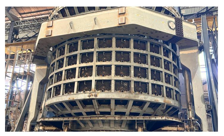
Mukand Limited has successfully manufactured its first-ever Coke Bucket and Carriage that ensures efficient transfer of hot coke from the coke oven to the Coke Dry Quenching (CDQ) system. CDQ is an advanced and environmentally friendly alternative to traditional wet quenching that significantly reduces CO2 emissions, conserves water, and enhances coke quality.
